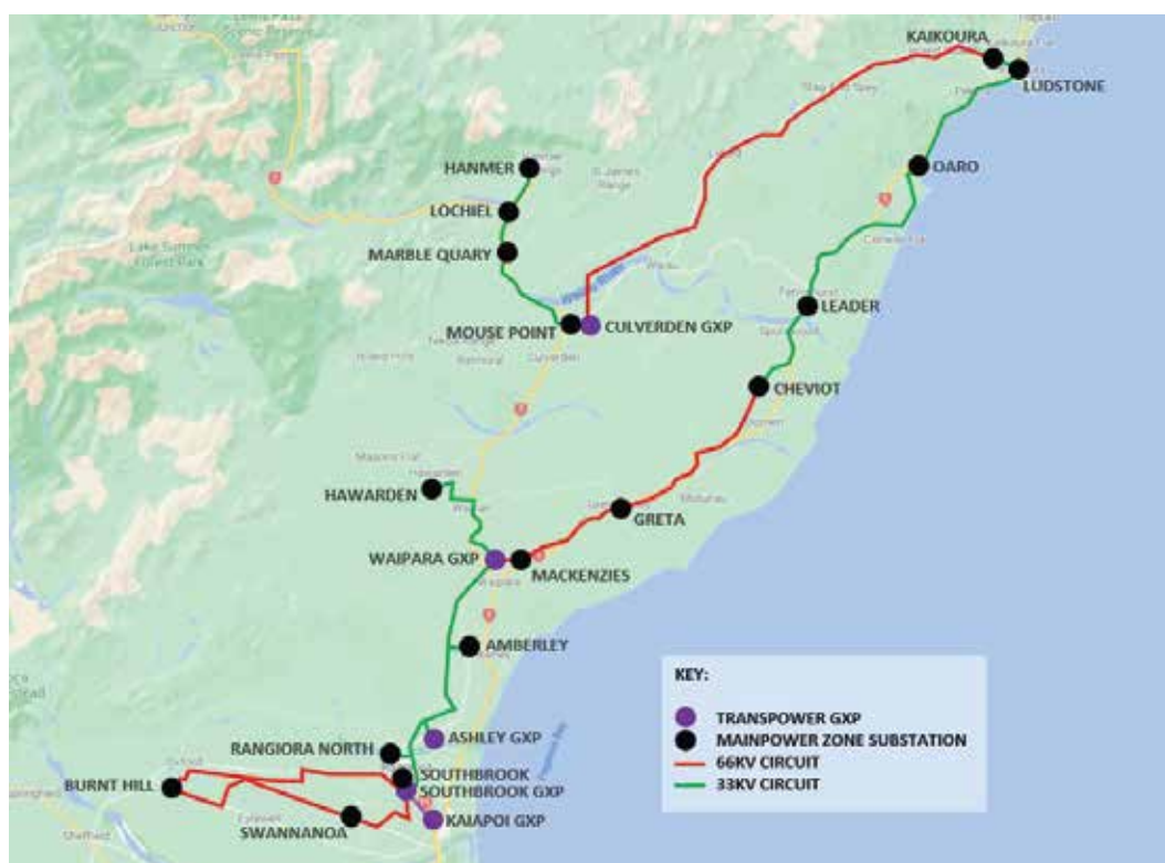
Figure 7.13: Zone Substation Locations
