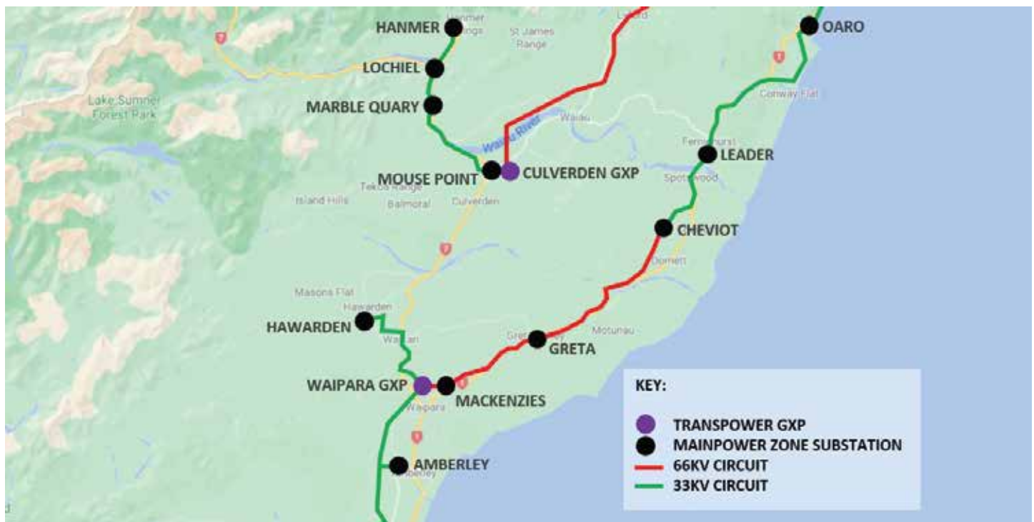
Figure 6.6: Hurunui Sub-Transmission Network (Existing)
