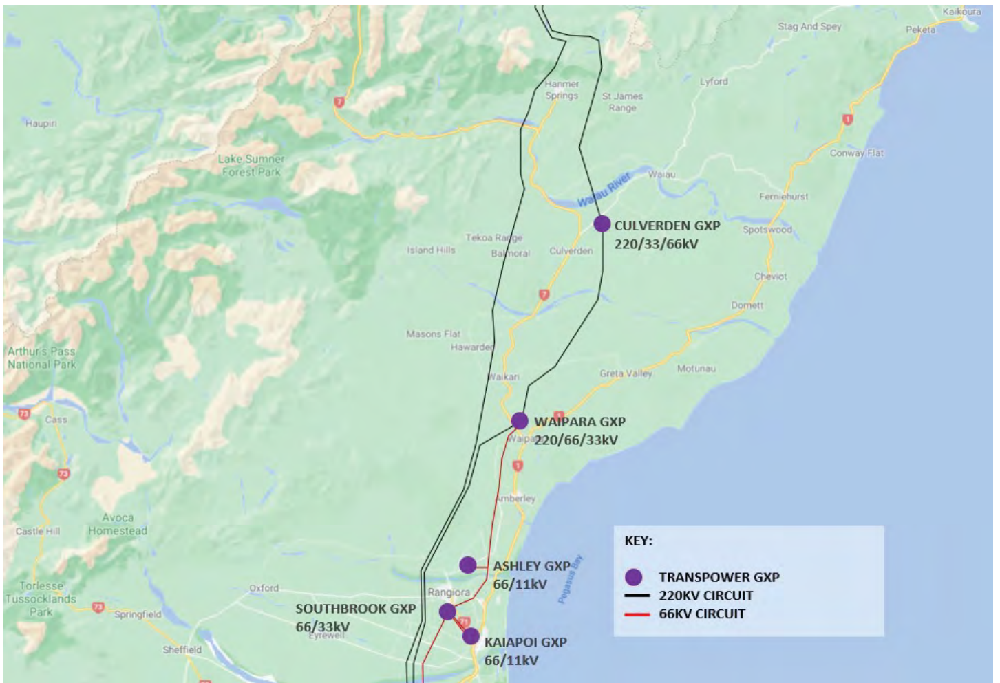
Figure 5.2: Transpower's North Canterbury Transmission Grid
