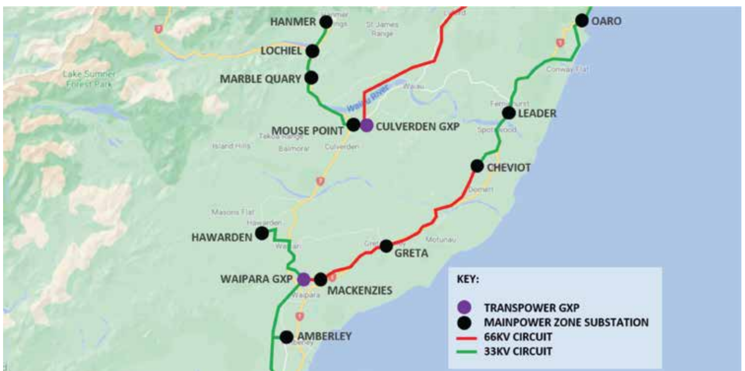
Figure 6.7: Hurunui sub-transmission network (existing)
