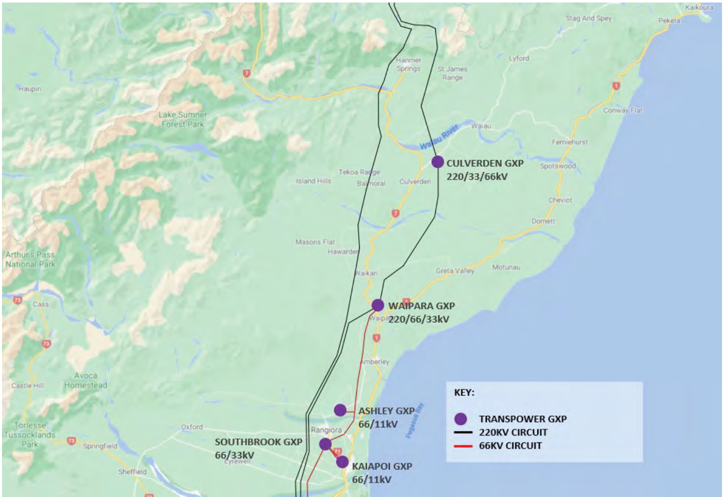
Figure 5.2: Transpower's North Canterbury transmission grid
