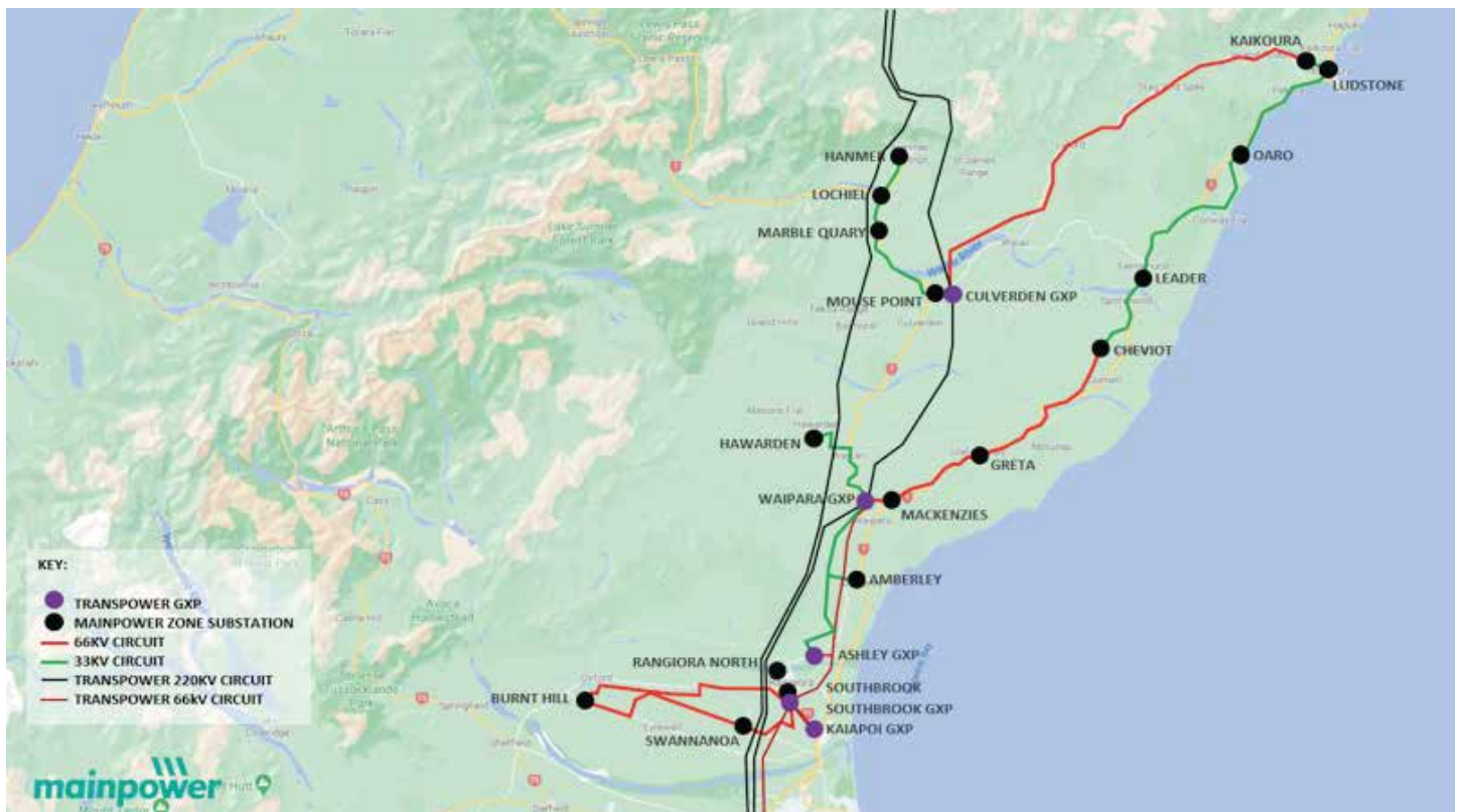
Figure 5.3: MainPower’s Sub-transmission Network
