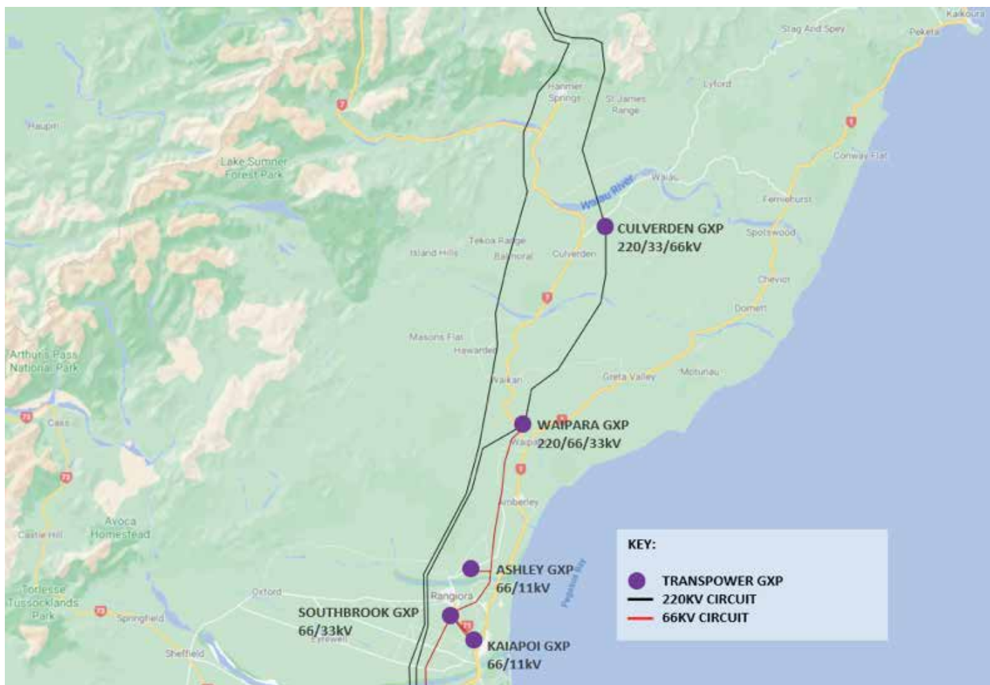
Figure 5.2: Transpower's North Canterbury Transmission Grid
